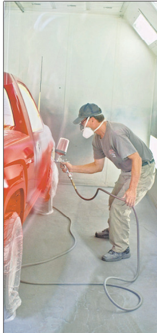
A Campbell Collision painter sprays newly mixed waterborne Victory Red paint onto a Dodge Dakota pickup in the paint booth. PHOTO BY DENYSE SMITH/DAILY PRESS & ARGUS
